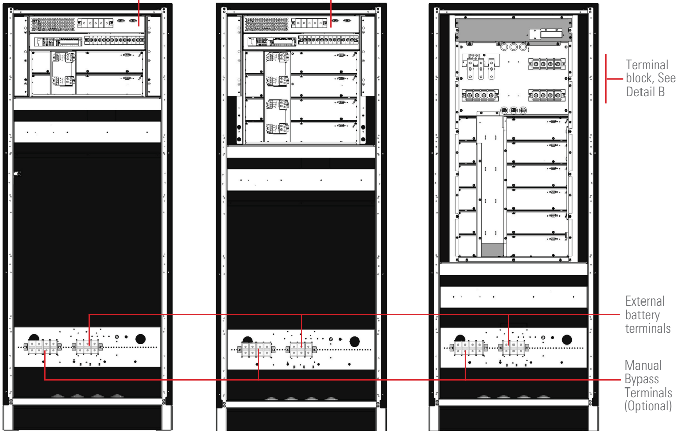
Fig. 4. Rear views of the 33U cabinet with protective cover removed for 2, 4 and 6 modules installed.
